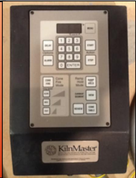
The KM1 Wall Mount Controller can upgrade just about any KilnSitter controlled kiln under 50Amps with a NEMA 6-50 or NEMA 15-50 plug to perform just like an automatic kiln. Just plug your kiln into the back of the controller, plug the controller into the wall outlet and install the thermocouple.
